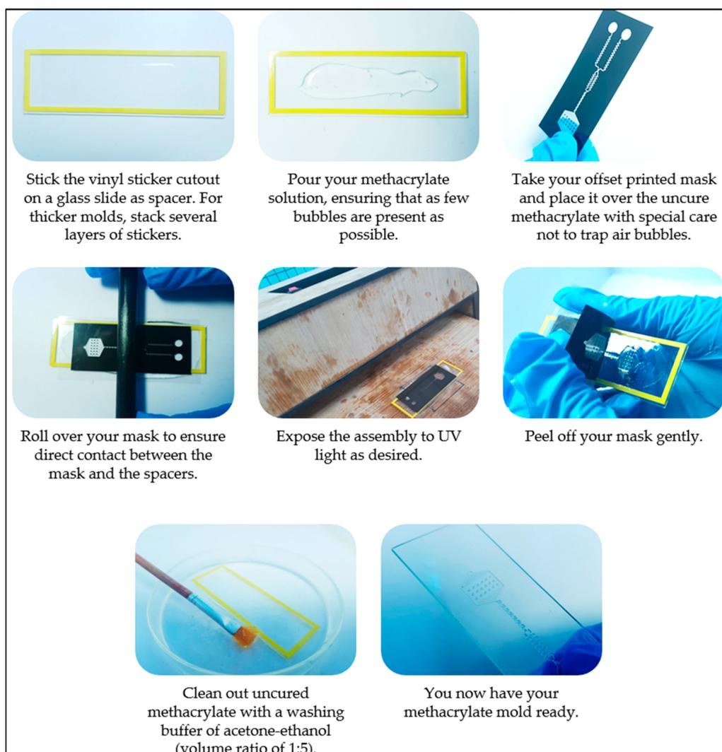
**Figure 1.** Photolithographic procedure.
