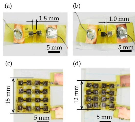
**Figure 4.** Photographic images of the fabricated devices. A single pair of TE generators in (a) the deployed state and (b) the folded state. Eight pairs of TE generators in (c) the deployed state and (d) the folded state.
