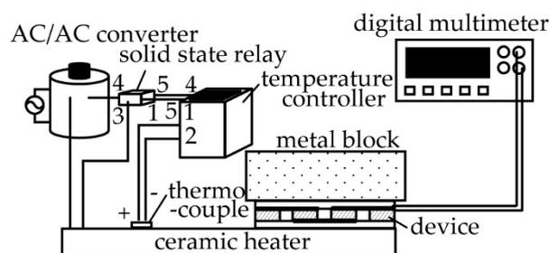
**Figure 3.** Experimental setup for measuring the output voltage of the flexible TE generator.
