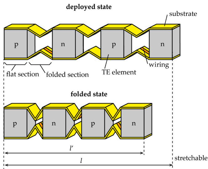
**Figure 1.** Stretchable substrate using origami-like folding deformation.
