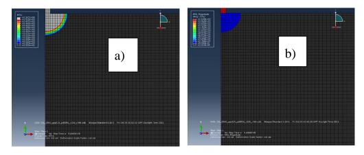
**Figure 3.** Electric force efficiency for a current intensity of 5.6 A: (a) erosion crater; (b) electric potential gradient.
