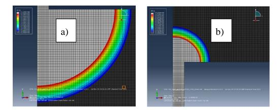
**Figure 2.** Shape of the erosion crater on the electrodes for a current intensity of 51.4: (**a**) workpiece; (**b**) tool.
