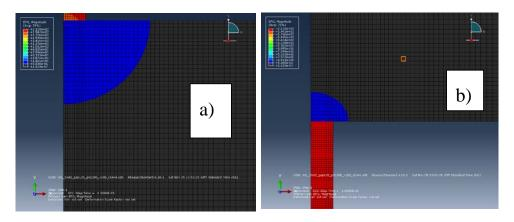
Figure 1. Electrical potential gradient for a current intensity of 51.4 A: (a) work piece; (b) Tool.
