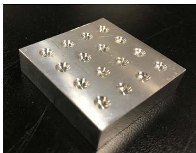
**Figure 6.** Mold for packaging MEMS pressure sensors.
