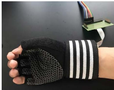
Figure 9. The wearable pulse wave monitoring system.
