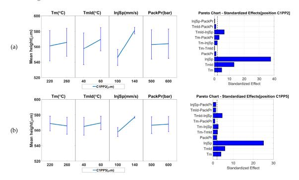
**Figure 12.** Influence of the IM process parameters on the measurands (pillar height) and possible product fingerprints from cavity: (a) C1PP2 (micro pillars far from the gate) and (b) C1PP5 (micro pillars near the gate). The figure presents the main effects. The error bars in the main effects plots represent the standard deviations from the respective measurand.
