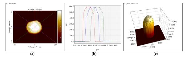
**Figure 8.** Pillar height measurement [20], (**a**) the four planes intersecting the middle of the pillar for the extraction of the cross-section profiles, (**b**) the four cross-section profiles of the pillar, and (**c**) the 3D representation of a pillar.
