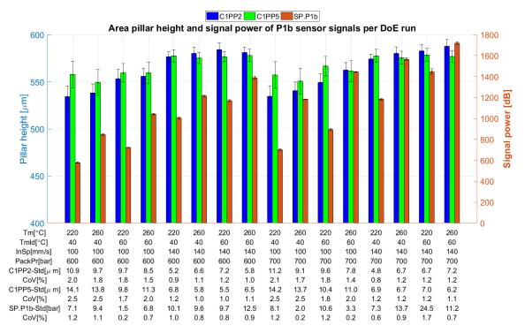
**Figure 15.** Values of the measurands in positions C1PP2 (far from the gate), C1PP5 (near the gate), and the average power of the signal originating from the piezoelectric pressure sensor *P1b* far from the gate in Cavity 1.
