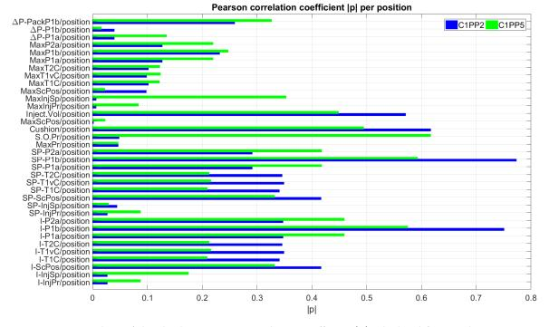
**Figure 16.** Values of the absolute Pearson correlation coefficient  $|\rho|$  calculated from each process fingerprint candidate with respect to the feature height in positions C1PP2 (far from the gate) and C1PP5 (near the gate) of Cavity 1. The process fingerprint candidates are listed in the y axis of the figure.
