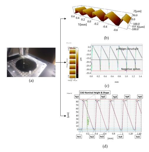
**Figure 9.** (a) Measurement of the R structure on a Keyence CLSM microscope. (b) SPIP 3D scan of position C2R551. (c) Cross-section profile extraction. In this scenario, the position C2R511 is used to portray the negative "spikes" caused by the replication of the burrs. (d) Illustration of a measurement procedure example for peak height ( $R_{height}$ ) on the profiles of position C2R551.
