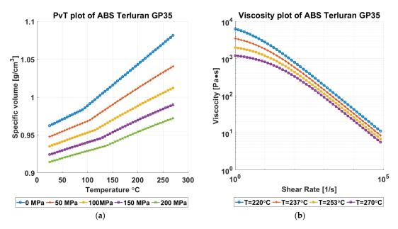
Figure 7. (a) PvT and (b) viscosity plots of material Styrolution Terluran GP-35 (ABS) [18].
