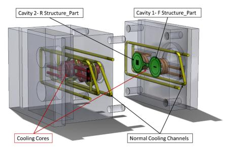
Figure 5. Mold geometry and cooling channels.
