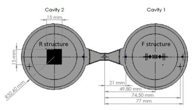
**Figure 2.** Structures of interest on full molded part. Cavity 1 includes the F structure, which is presented in more detail in Figure 3. Cavity 2 includes the R structure, which is presented in more detail in Figure 4. The F structure is in Cavity1 and the R structure is in Cavity 2.
