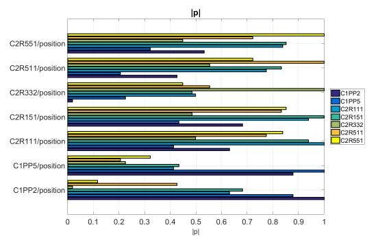
**Figure 14.** Values of the absolute Pearson correlation coefficient  $|\rho|$  calculated from each possible combination of the seven measurands from Cavity 1 and 2. A perfect correlation ( $|\rho| = 1$ ) exists only for combinations of the same dataset.
