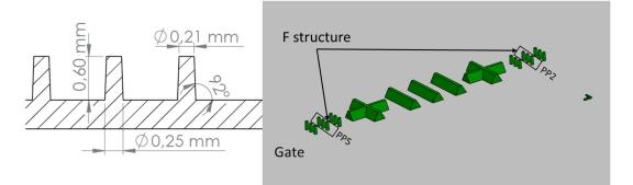
**Figure 3.** Cavity 1, F structure. Micro pillars used to assess part quality and process fingerprints are marked on the figure. PP5 indicates micro features near the gate while PP2 indicates micro features far from the gate.
