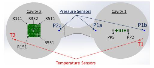
**Figure 6.** Measurement positions of structures and sensor position on full molding. In this case, the sensor positions are shown in the front side of the molding for easier association of the feature measurement to the sensor recordings. The F structure is in Cavity1 and the R structure is in Cavity 2.
