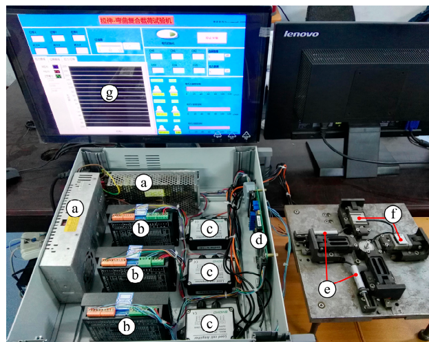
Figure 5. Loading test system diagram. (a) Power supply; (b) Motor control; (c) Signal amplifier; (d) Data acquisition card; (e) Displacement transducer; (f) Force transducer; (g) Upper computer.
