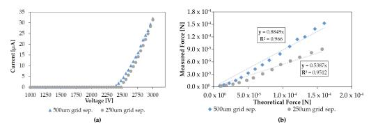
**Figure 8.** (a) Changing the grid wire separation from 500  $\mu$ m to 250  $\mu$ m had an insignificant effect on discharge characteristics with a bare wire at a 1 mm gap distance; (b) Decreasing the wire separation changed the loss factor by over 30%. Because there is no change in IV characteristics the increased losses can presumably be attributed to increased drag.
