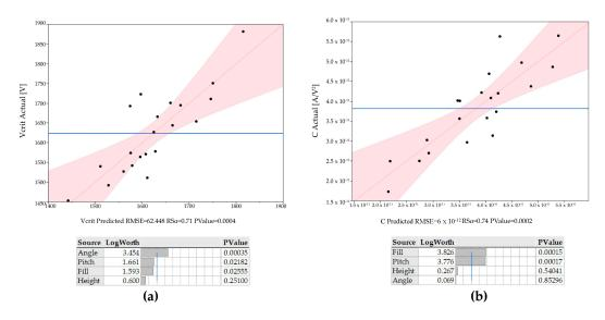
**Figure 5.** Response models generated by least squares regression analysis of the 21 run dataset. A p value below 0.05 generally represents a statistically significant factor (rejection of the null hypothesis). (a) The regression model for corona inception voltage; (b) The regression model for C coefficient.
