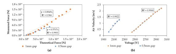
**Figure 10.** (a) Changing the electrode gap distance from 1 mm to 500  $\mu$ m with all else held constant increased loss factor by over 30%. Test performed with a bare wire, a 500  $\mu$ m grid wire separation, and a 25  $\mu$ m wire width; (b) Measured outlet air velocity versus applied voltage for the two electrode gap distances. As expected by combining Equations (1) and (2) with the mass flow equation, the voltage-velocity relationship is linear above the corona onset voltage.
