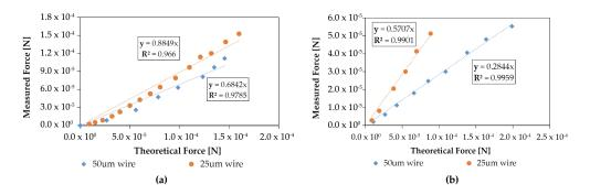
**Figure 9.** Both of these figures are for 500  $\mu$ m grid wire separations with a bare wire as the emitter electrode. (a) Changing the grid wire width from 25  $\mu$ m to 50  $\mu$ m at a 1 mm electrode gap increased loss factor by about 20% without a significant effect on discharge current; (b) Changing the grid wire width from 25  $\mu$ m to 50  $\mu$ m at a 0.5 mm electrode gap increased loss factor by about 19% without a significant effect on discharge current.
