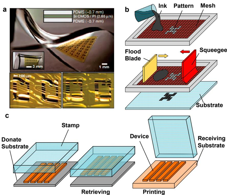
**Figure 4.** (a) Stretchable integrated circuits fabricated based on CMOS technology (Reprinted with permission from Ref. [26] Copyright 2008 American Association for the Advancement of Science); (b) a schematics of the screen printing process; and (c) a schematics of the transfer printing process.
