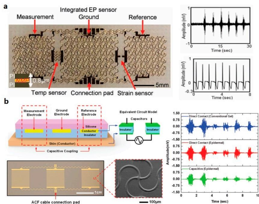
**Figure 5.** Examples of skin sensors for biopotential measurement: (a) biopotential measurement using skin-contacted metallic electrodes (Reprinted with permission from Ref. [91] Copyright 2013 John Wiley and Sons); and (b) an epidermal electronic system (EES) with a capacitive sensor for electrophysiological (EP) measurement (Reprinted with permission from Ref. [18] Copyright 2014 John Wiley and Sons).
