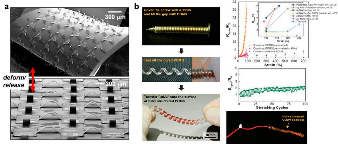
**Figure 2.** Examples of out-of-plane structures with high stretchability: (a) SEM images of arrays of complementary metal-oxide semiconductor (CMOS) inverters with spatially buckled bridges (Reprinted with permission from Ref. [29] Copyright 2008 National Academy of Sciences); and (b) helical-structured copper nanowire (CuNW)-based electrodes (Reprinted with permission from Ref. [41] Copyright 2014 Nature Publishing Group).
