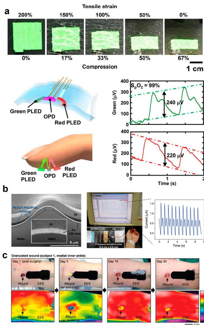
**Figure 10.** Skin sensors used for other sensing applications: (a) a skin sensor that can measure oxygen concentration of blood (Reprinted with permission from Ref [177] Copyright 2016 The Authors); (b) a stretchable resistive pressure sensor (Reprinted with permission from Ref [182] Copyright 2014 John Wiley and Sons); and (c) an epidermal electronics system that can monitor cutaneous wound healing (Reprinted with permission from Ref. [180] Copyright 2014 John Wiley and Sons).
