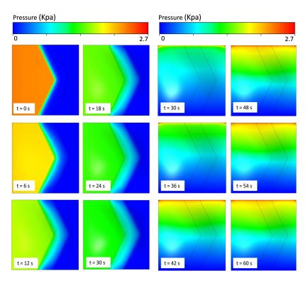
**Figure 8.** Pressure distribution for various time steps for L/W = 0.65 model in upper surfaces and lower surfaces of membrane in microvalves.
