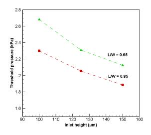
**Figure 13.** Opening threshold pressure of microvalve for various inlet region heights for L/W = 0.65 and 0.85 models.
