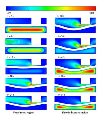
**Figure 10.** Velocity contours' fields and streamlines for various time steps for L/W = 0.65 model in the A-A' cross-sectional plane.
