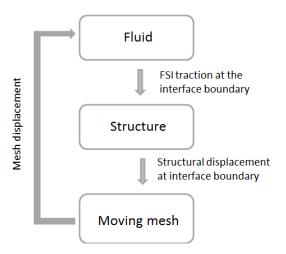
Figure 4. Schematic diagram of fluid-structure interaction.
