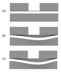
**Figure 5.** Initial and deformed stages of microvalve mesh in A-A' cross-sectional plane: (**A**) Initial state of the microvalve. (**B**,**C**) Microvalve membrane deflected against pressure developed by fluid flow in the source region.
