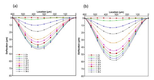
**Figure 11.** Deformation of membrane in the A-A' cross-sectional plane is shown in various time steps at an input flow rate of 8  $\mu$ L/min are used in both L/W-ratio models (**a**) L/W = 0 and (**b**) L/W = 0.65 model.
