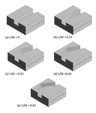
Figure 2. (a-e) Shows that various shapes of microvalve fluid domain model illustrated with length/width (L/W) ratio.
