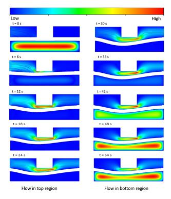
**Figure 9.** Velocity contours' fields and streamlines for various time steps for L/W = 0 model in the A-A' cross-sectional plane.
