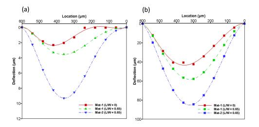
**Figure 12.** Deformation of membrane in the A-A' cross-sectional plane is shown in various material properties at an input flow rate of 8  $\mu$ L/min are used in both L/W-ratio models (**a**) L/W = 0 and (**b**) L/W = 0.65 model.
