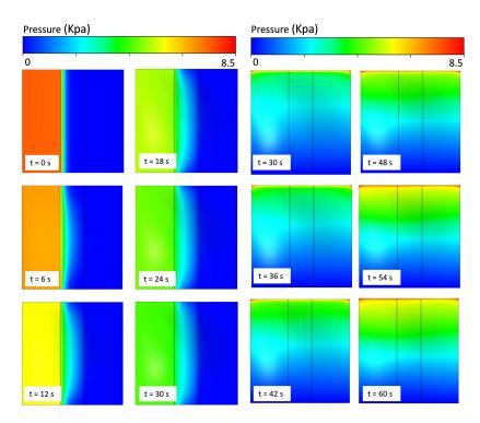
**Figure 7.** Pressure distribution for various time steps for L/W = 0 model in upper surfaces and lower surfaces of membranes in microvalves.
