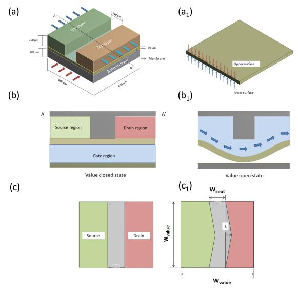
**Figure 1.** Normally closed (NC) microvalves: (a) 3D microvalve, and dimensions of top and bottom actuation chamber; ( $a_1$ ) Structural membrane; ( $b,b_1$ ) Cross-sectional view of microvalves open and closed structural domain in A-A' position, and source, drain and gate regions of the valve. Open and closed states of microvalve: ( $c,c_1$ ) top view of microvalve, and measurement of different vertex positions.
