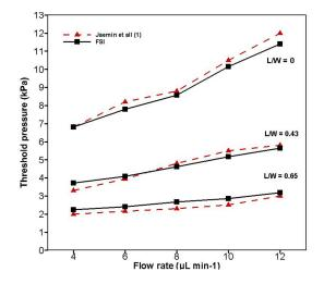
**Figure 6.** Comparison of experimental results with fluid-structure interaction (FSI) results for changes in opening threshold pressure against change in flow rate.
