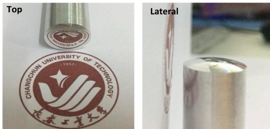
**Figure 11.** Convex spherical surface topography of titanium alloy machined by a non-resonant three-dimensional elliptical vibration cutting (3D-EVC) apparatus ( $f_{3D} = 50$  mm/min,  $S = 50$  mm/min,  $A = 7$   $\mu$ m,  $D = 1$   $\mu$ m and  $F = 0.2$  mm $\cdot$ min $^{-1}$ ). (left) Top view; (right) Lateral view.
