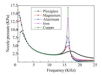
**Figure 16.** The frequency response curves of the nozzle pressure of the micro-jet (shell with different materials).
