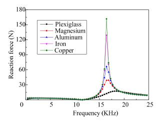
**Figure 18.** The frequency response curves of the reaction force of the vibrator when selecting shells with different acoustic impedance.
