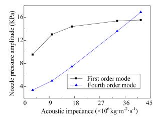
Figure 17. The amplitudes of the nozzle pressure vary with different acoustic impedance of the shell.
