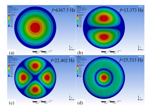
**Figure 4.** The mode shapes and the corresponding resonant frequencies of the vibrator when the cavity is filled with air: (**a**) first-order mode with the resonant frequency as 6367.5 Hz; (**b**) second-order mode with the resonant frequency as 13,373 Hz; (**c**) third-order mode with the resonant frequency at 22,402 Hz; and (**d**) fourth-order mode with resonant frequency at 25,533 Hz.
