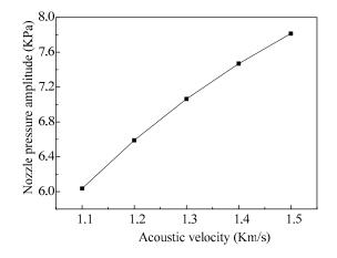
Figure 12. The amplitudes of the nozzle pressure vary with different acoustic velocity of the fluids.
