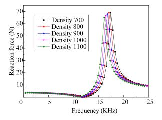
Figure 8. The frequency response curves of the reaction force of the vibrator when ejecting fluids with different densities.
