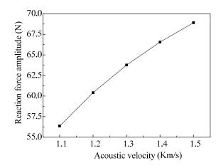
Figure 14. The amplitudes of the reaction force vary with different acoustic velocities of the fluid.
