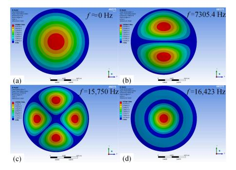
**Figure 5.** The mode shapes and the corresponding resonant frequencies of the vibrator when the cavity is filled with fluid: (**a**) first-order mode with the resonant frequency as close to 0 Hz; (**b**) second-order mode with the resonant frequency as 7305.4 Hz; (**c**) third-order mode with the resonant frequency as 15,750 Hz; and (**d**) fourth-order mode with the resonant frequency as 16,423 Hz.
