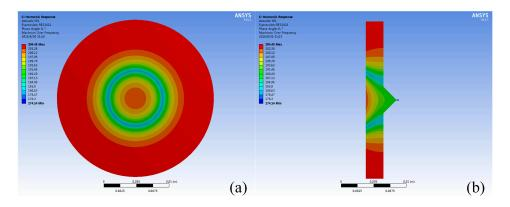
**Figure 2.** The acoustic pressure distribution in the fluid field of the piezoelectric micro-jet: (**a**) the global state of the pressure distribution; and (**b**) the cross-section diagram of the pressure distribution.
