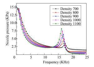
Figure 6. The frequency response curves of the nozzle pressure of the micro-jet (fluid with different densities).
