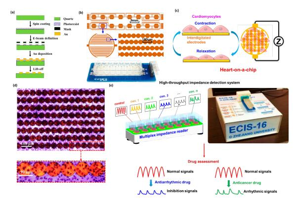
**Figure 1.** Establishment of heart-on-a-chip for drug assessment. (a) The fabrication of interdigitated electrodes (IDEs); (b) The IDEs layout and image of device; (c) Schematics of heart-on-a-chip with IDEs and impedance detection method; (d) The Diff-Quik staining images of cardiomyocytes on the device; (e) High-throughput impedance detection system for drug assessment using beating characteristics.
