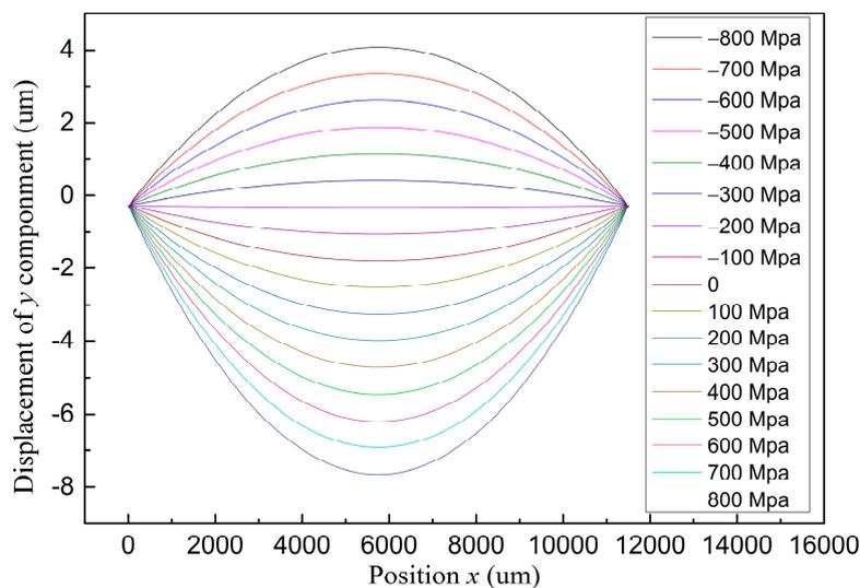
**Figure 4.** Displacement profiles of  $y$  component of the multilayer thin films under intrinsic stresses of  $\text{SiN}_x$  film ranging from  $-800$  MPa compressive stress to  $800$  MPa tensile stress, with stress increment of  $100$  MPa.
