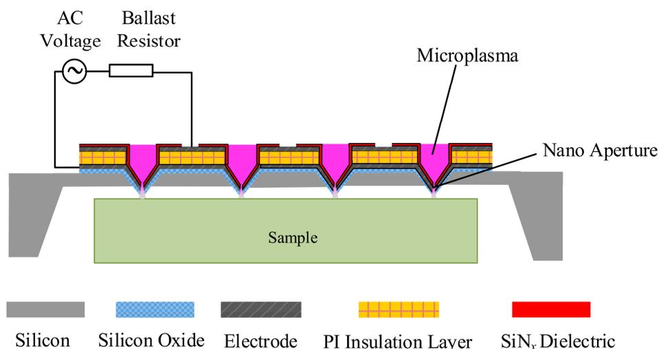
**Figure 1.** Schematic diagram of the inverted pyramid micro dielectric barrier discharge (MDBD) array for maskless nanoscale etching.
