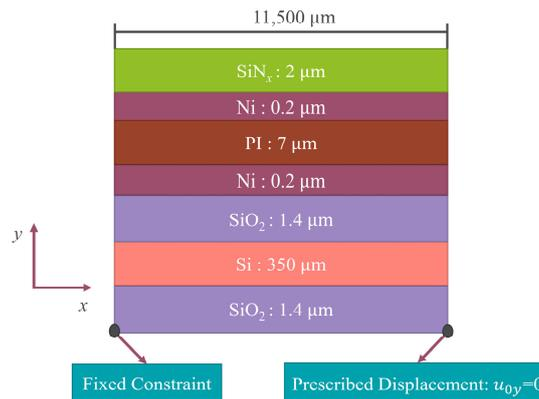
**Figure 2.** Two-dimensional plane stress approximation geometric model for MDBD device.
