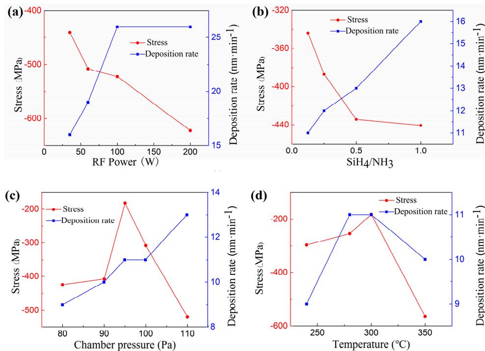
**Figure 5.** Influence of some of the key deposition parameters of the process: (a) RF power; (b) SiH<sub>4</sub>–NH<sub>3</sub> flow ratio; (c) Chamber pressure; (d) Temperature, with the intrinsic stress level and deposition rate. The equipment used here was PECVD (PD-220, SAMCO).
