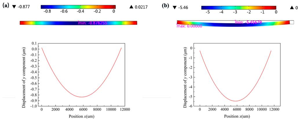
**Figure 3.** Displacement profiles of  $y$  component of the multilayer thin films. (a) Before deposition of  $\text{SiN}_x$ ; (b) After deposition of  $\text{SiN}_x$  film by plasma enhanced chemical vapor deposition (PECVD) with the original recipe (Plasma System100, Oxford Instruments).
