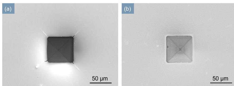
**Figure 6.** SEM images of inverted pyramid MDBD device. (a) After deposition of 2 μm-thick-SiN<sub>x</sub> by original recipe of PECVD (Plasma System100); (b) After deposition of 2 μm-thick-SiN<sub>x</sub> by optimized recipe of PECVD (PD-220, SAMCO).
