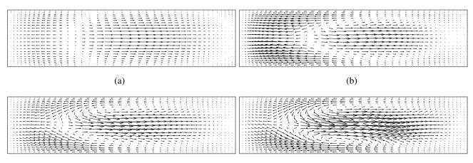
Figure 4. Cross-sectional velocity vectors at z = 0.25L, where L is the length of one geometric period of the channel with  $\alpha = 1$  and  $\beta = 1/3$ . (a) Re = 10, (b) Re = 30, (c) Re = 50 and (d) Re = 70.
