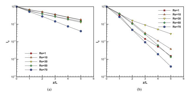
Figure 10. Effect of the Reynolds number on the intensity of segregation at a down-channel position z = 5L.
