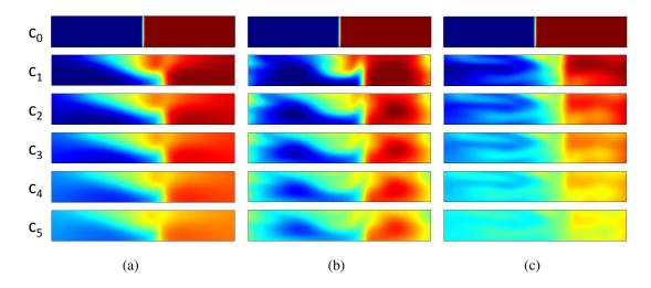
Figure 8. Evolution of the concentration in the mixer with  $\alpha=1$  at the three Reynolds numbers: (a) Re = 1, (b) Re = 30 and (c) Re = 70.
