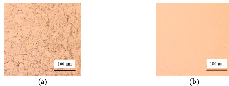
Figure 12. The influence of electrolyte flow rate on the surface quality. (a) 460 mL/min; (b) 300 mL/min.
