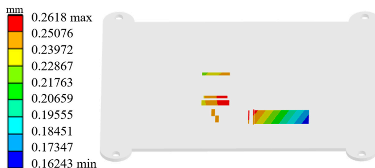
Figure 4. Z-direction deformation contour at critical locations on the base of the laser diode array beam combining module.
