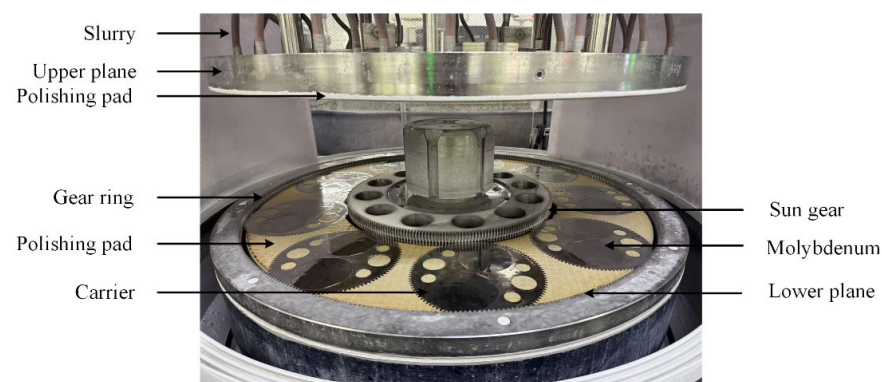
Figure 1. Double-sided chemical mechanical polishing system.
