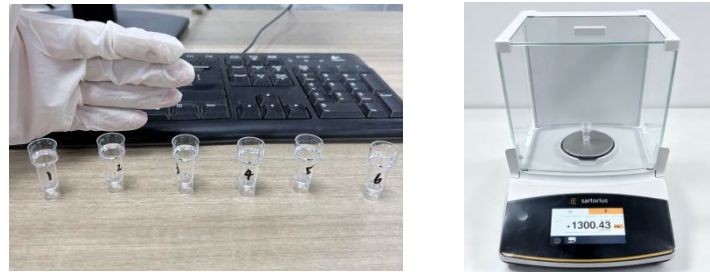
Figure 4. Tared sample cups and gravimetric measurement.
