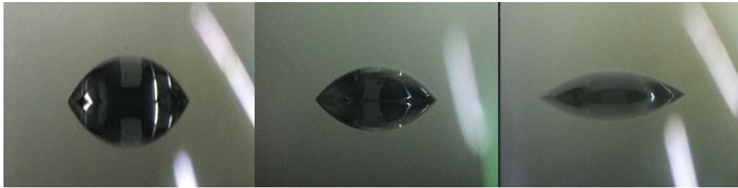
Figure 7. Three types of contact angle effects.
