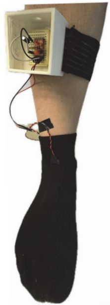
Figure 17. Sock with piezoelectric sensors and circuitry used to collect energy while walking.
