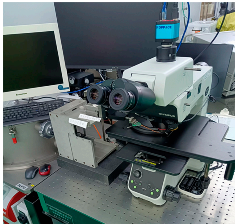
Figure 13. Testing equipment consisting of Olympus MX63 optical microscope, custom-designed probe holder, and video recording system.
