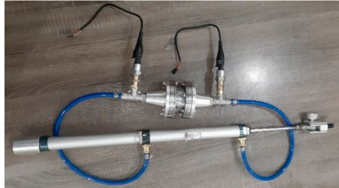
Figure 4. MR valve and double-ended cylinder setup.
