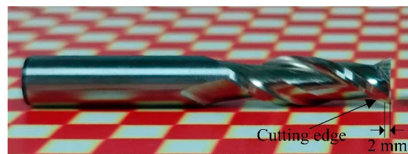
Figure 20. The two-flute keyway milling cutter.
