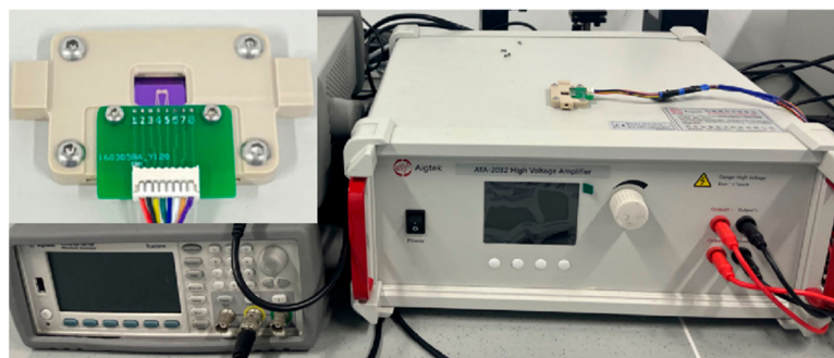
Figure 7. Microfluidic ink cartridge containing the DEP chip, along with the signal generator and high-voltage amplifier equipment for applying DEP forces.
