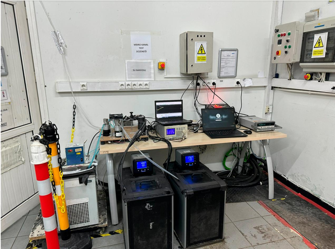
**Figure 6.** Secondary loop water baths, DAQ system, power supplies and electronic control units of the experimental setup.
