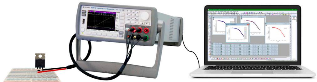
Figure 2. Schematic representation of setup for  $I$ - $V$  transfer characteristics measuring.
