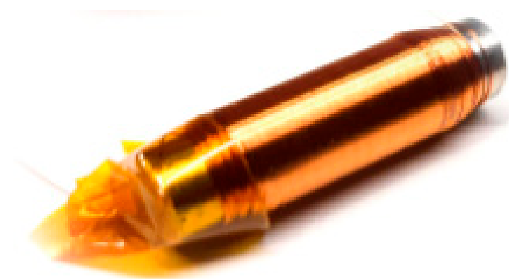
Figure 30. Torque coils made in-house.
