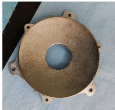
Figure 18. Primary mirror modified by Ni-P.
