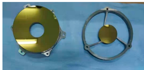
Figure 21. Primary and secondary mirrors after gold-plating.
