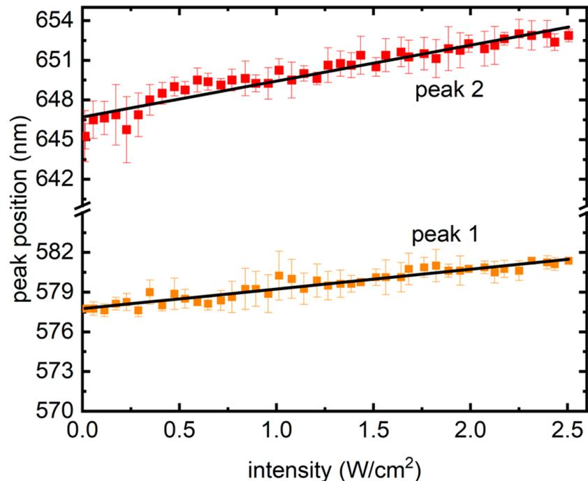
**Figure 5.** Redshift from the two peaks as the intensity of excitation grew. The symbols represent the average of peak wavelength positions from the four samples, whereas the error bars present their standard deviations. Solid lines are linear fits.
