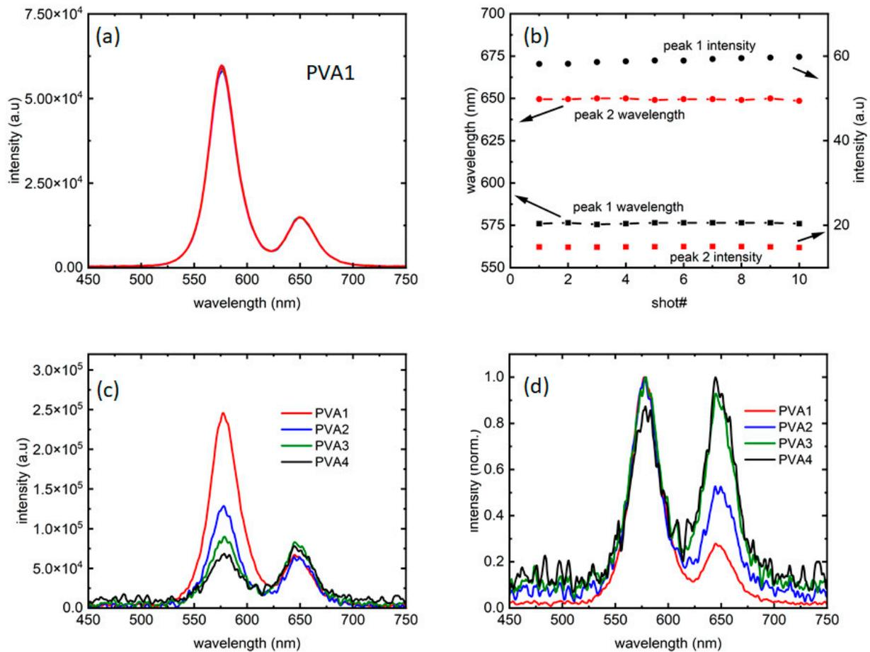
**Figure 2.** (a) A total of 10 traces collected over a period of 1 min show the repeatability of the data with each color presenting one measurement (also referred to as a “shot”). (b) Peak 1 and 2 emission wavelengths, along with the corresponding intensities from (a) with the arrows showing the axes used. (c) Intensity comparison of the four samples studied and (d) their normalized versions compared to probe any difference in linewidths.
