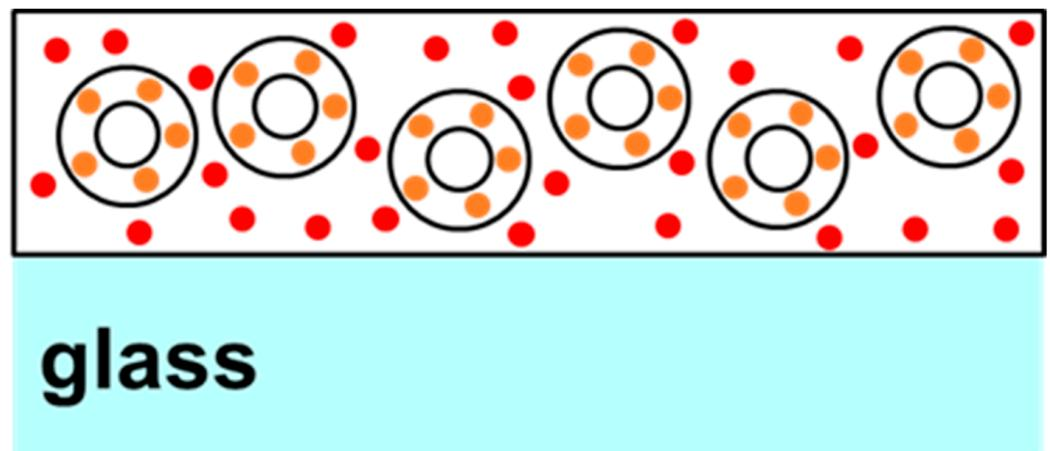
**Figure 1.** Structure of two-phase two-QD samples showing orange QDs bound in the shells of silica microparticles and red QDs dispersed in the surrounding PVA polymer.
