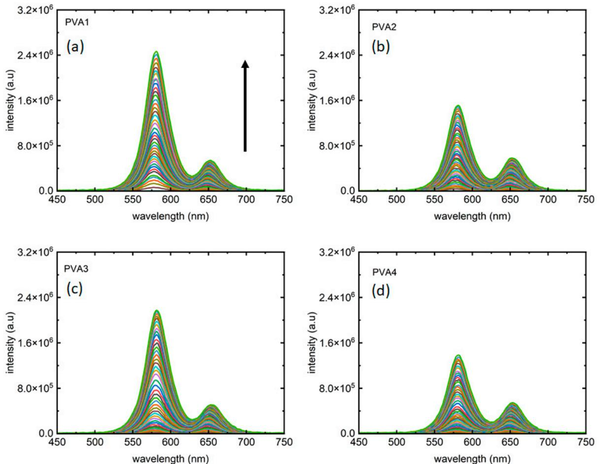
**Figure 3.** Fluorescence from the two-phase materials as the excitation laser intensity varied from 0–2.5 W/cm<sup>2</sup>. (a) PVA1, (b) PVA2, (c) PVA3, and (d) PVA4, respectively, present PL from the four samples, with each color corresponds to an excitation intensity for which the PL has been collected. The arrow shows the direction of increment of excitation laser intensity in all plots.
