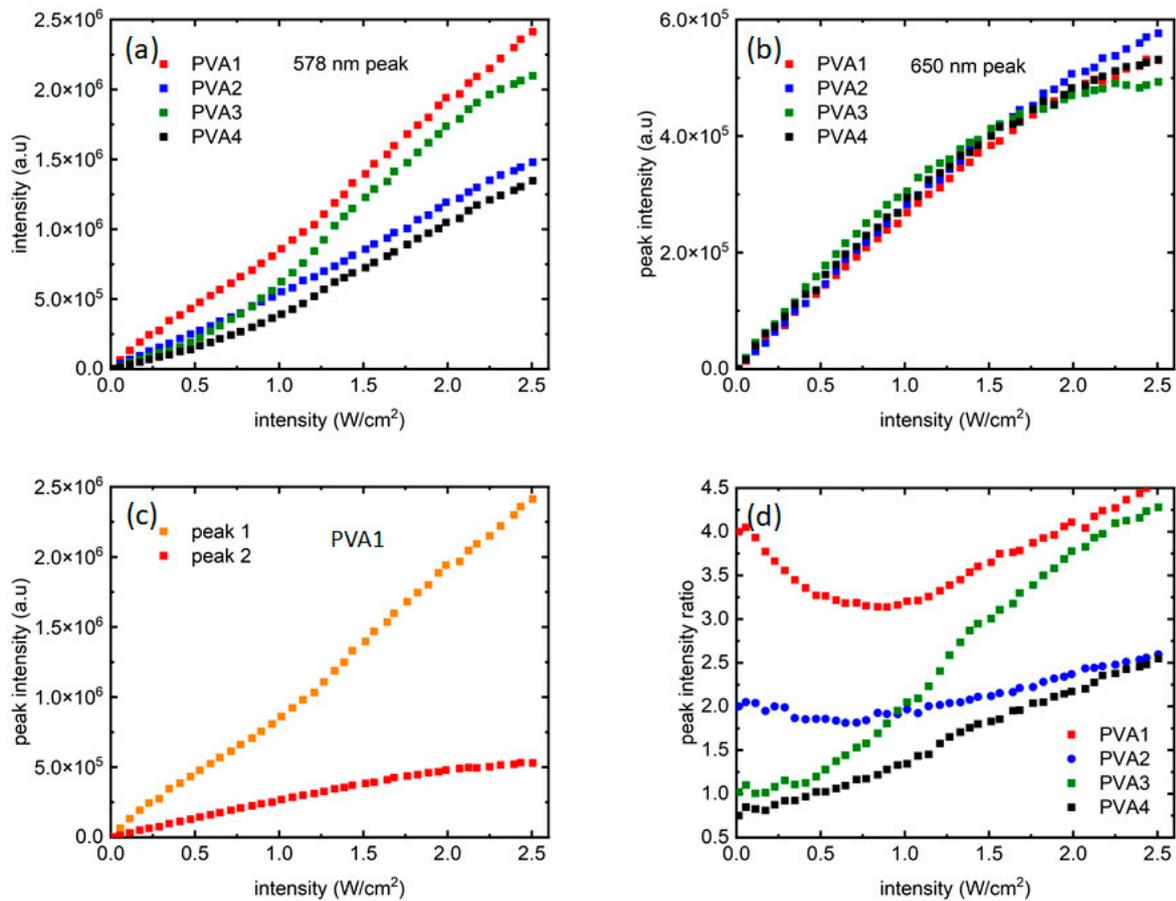
**Figure 4.** Growth of fluorescence intensities from the two QDs as the excitation laser intensity varied from 0–2.5  $\text{W/cm}^2$ : (a,b) present intensity growth of peak 1 and peak 2, respectively; (c) presents a comparison between peak 1 and peak 2 growth for PVA1. (d) Ratio of the two peak intensities as the laser intensity increased.
