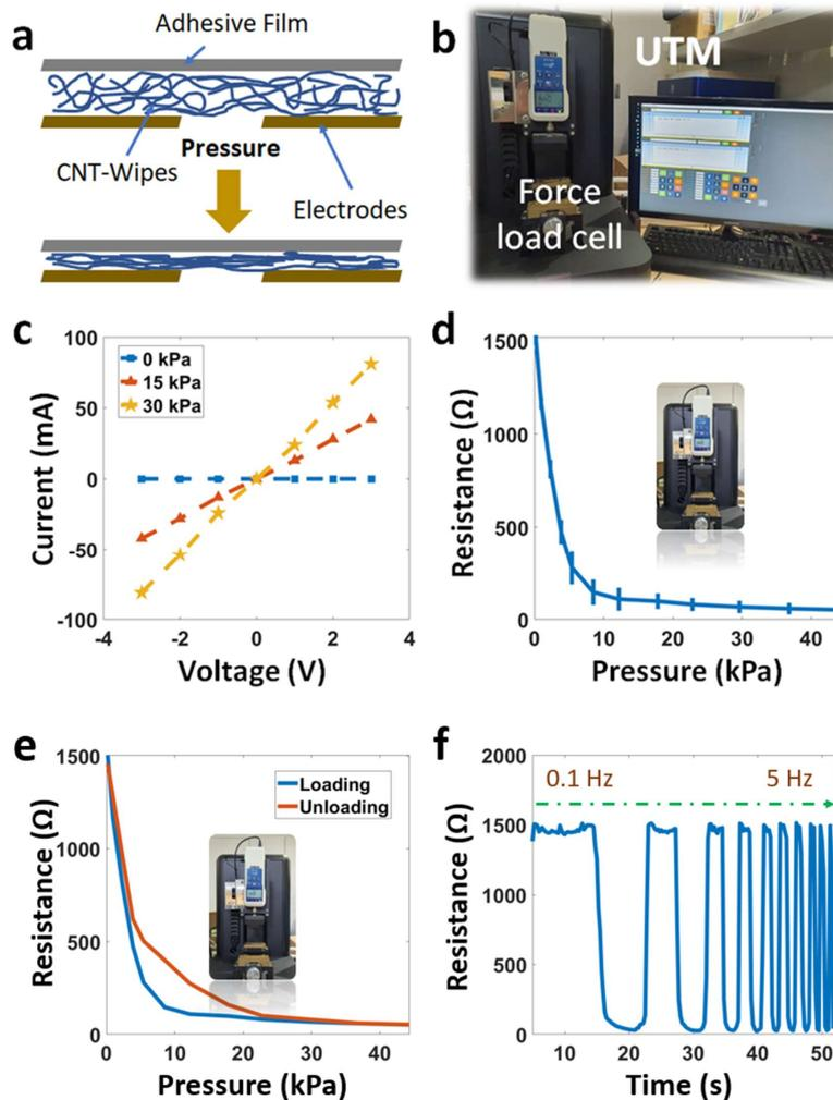
**Figure 3.** Characteristics of the sensor: (a) working principle, (b) universal testing machine, (c) current–voltage graphical curves, (d) resistance change under pressure, (e) hysteresis, and (f) resistance change at different frequencies.
