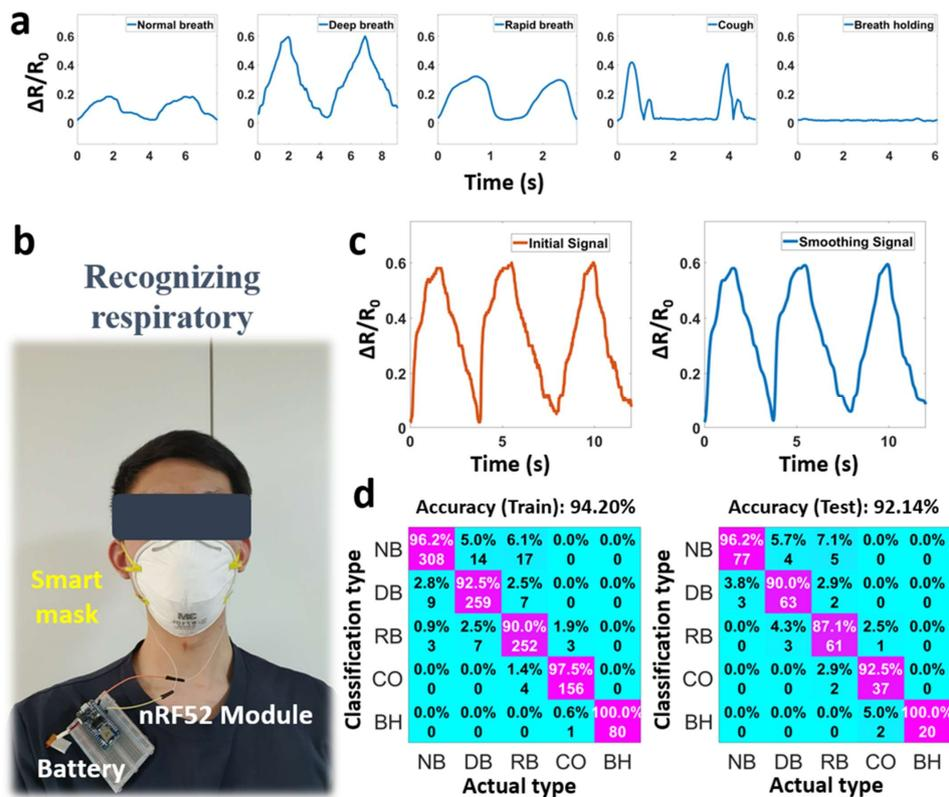
Figure 6. Respiratory monitoring system, consisting of (a) different breathing signals, (b) smart mask for recognizing respiratory, (c) initial and smoothing signal, and (d) confusion matrices.
