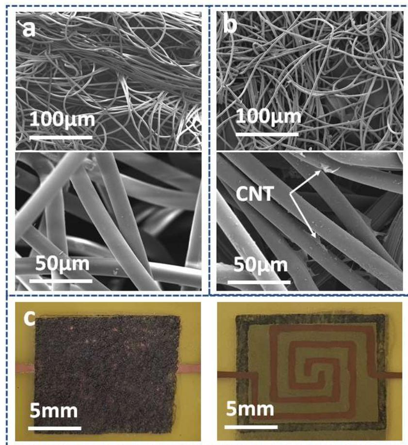
**Figure 2.** Scanning electron microscope images of the sensor: (a) sensing layer at 100  $\mu\text{m}$  and 50  $\mu\text{m}$  before dipping in CNTs, (b) sensing layer at 100  $\mu\text{m}$  and 50  $\mu\text{m}$  after dipping in CNTs, and (c) assembled sensor at the top view and bottom view.
