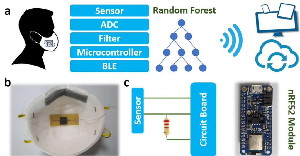
**Figure 5.** (a) Respiration checking with the embedded system, (b) smart mask with the flexible sensor, and (c) signal processing board with nRF52 module.
