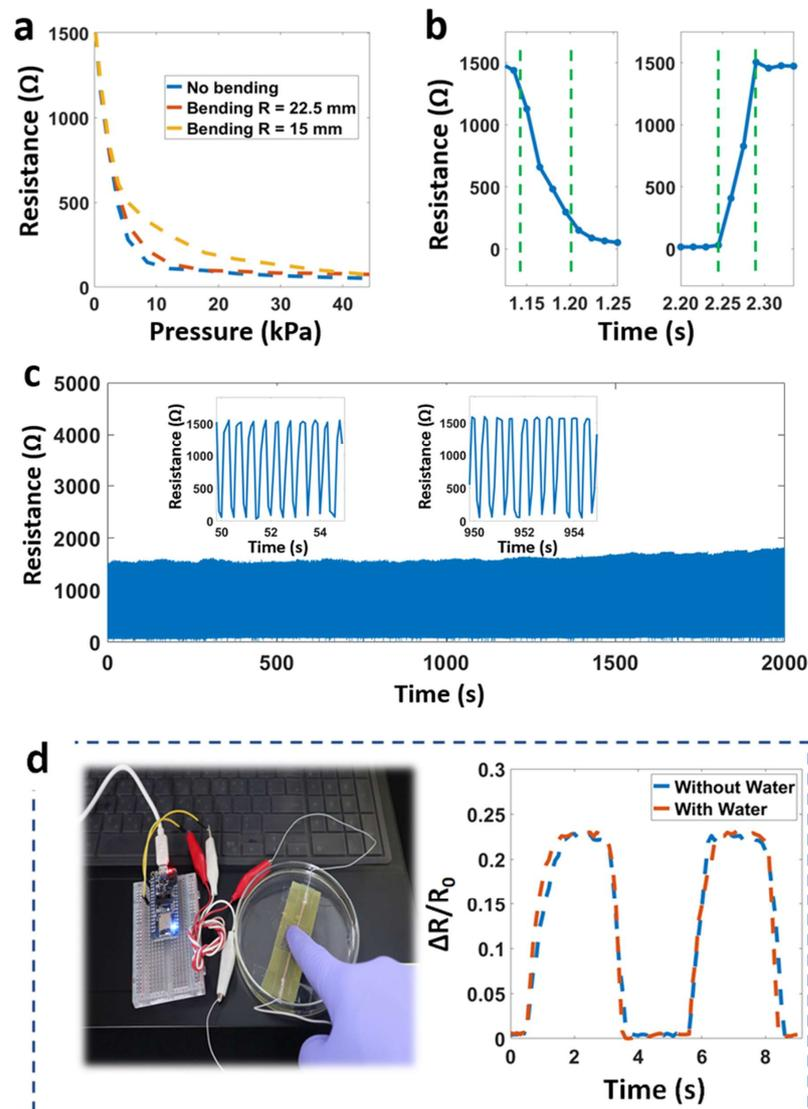
**Figure 4.** (a) Resistance change at different bending radii, (b) response and recovery times, (c) durability under loading/unloading cycles, and (d) working when dipped under water.
