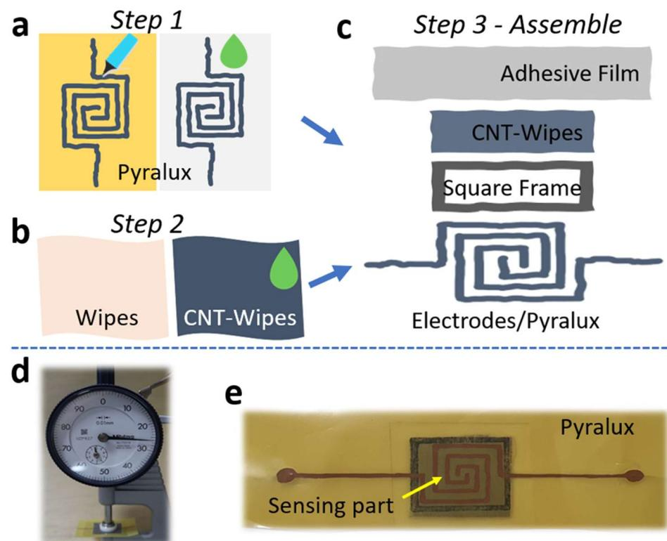
**Figure 1.** Manufacturing process of the flexible pressure sensors, consisting of (a) preparing the electrode layer, (b) preparing the sensing layer, (c) assembling sensor, (d) thickness of the sensor, and (e) real image of the final flexible sensor.
