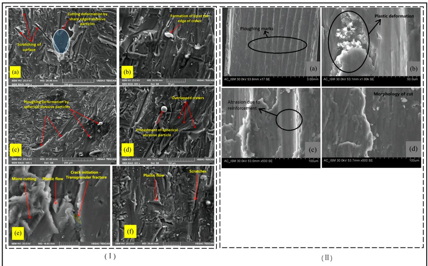
**Figure 5.** (I) Deformation mechanism involved in AZ91 magnesium alloy [35,36]. (a–d) indicates cutting deformation, ploughing deformation and plastic deformation of the material, (e,f) indicates micro-cutting, crack initiation and plastic flow in materials. (II) SEM image of the machined surface [37]. (a) ploughing mark,(b) plastic deformation; (c) abrasion; (d)morphology of cut.
