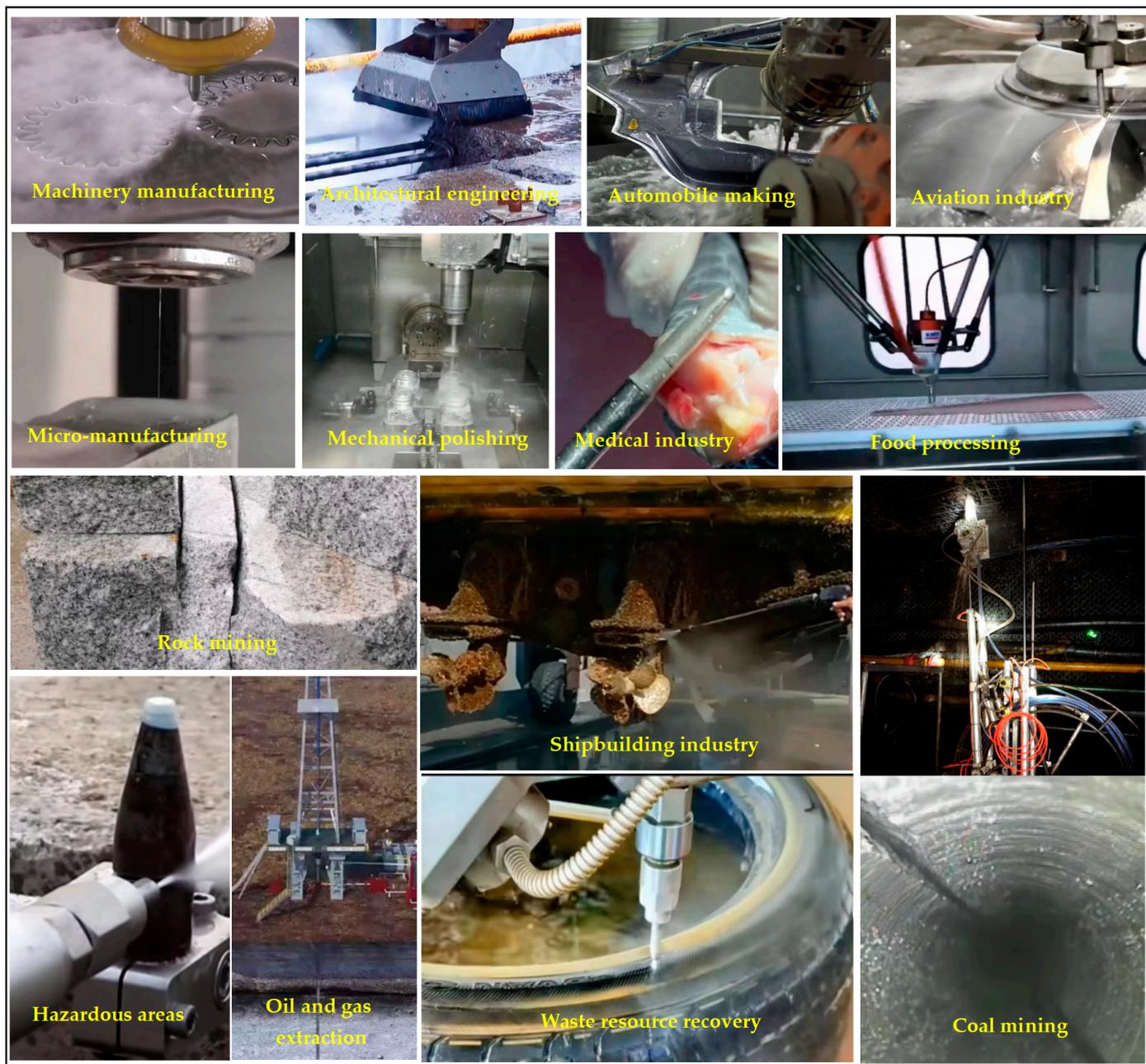
**Figure 12.** Application fields of abrasive water jets.
