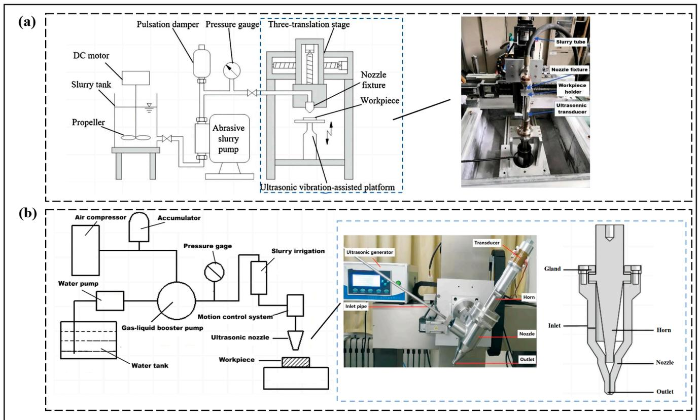
**Figure 13.** Effect of process parameters on surface roughness of different cutting areas: (a) ultrasonic vibrations applied to the workpiece [134]; (b) ultrasonic vibrations applied to the nozzle [135].
