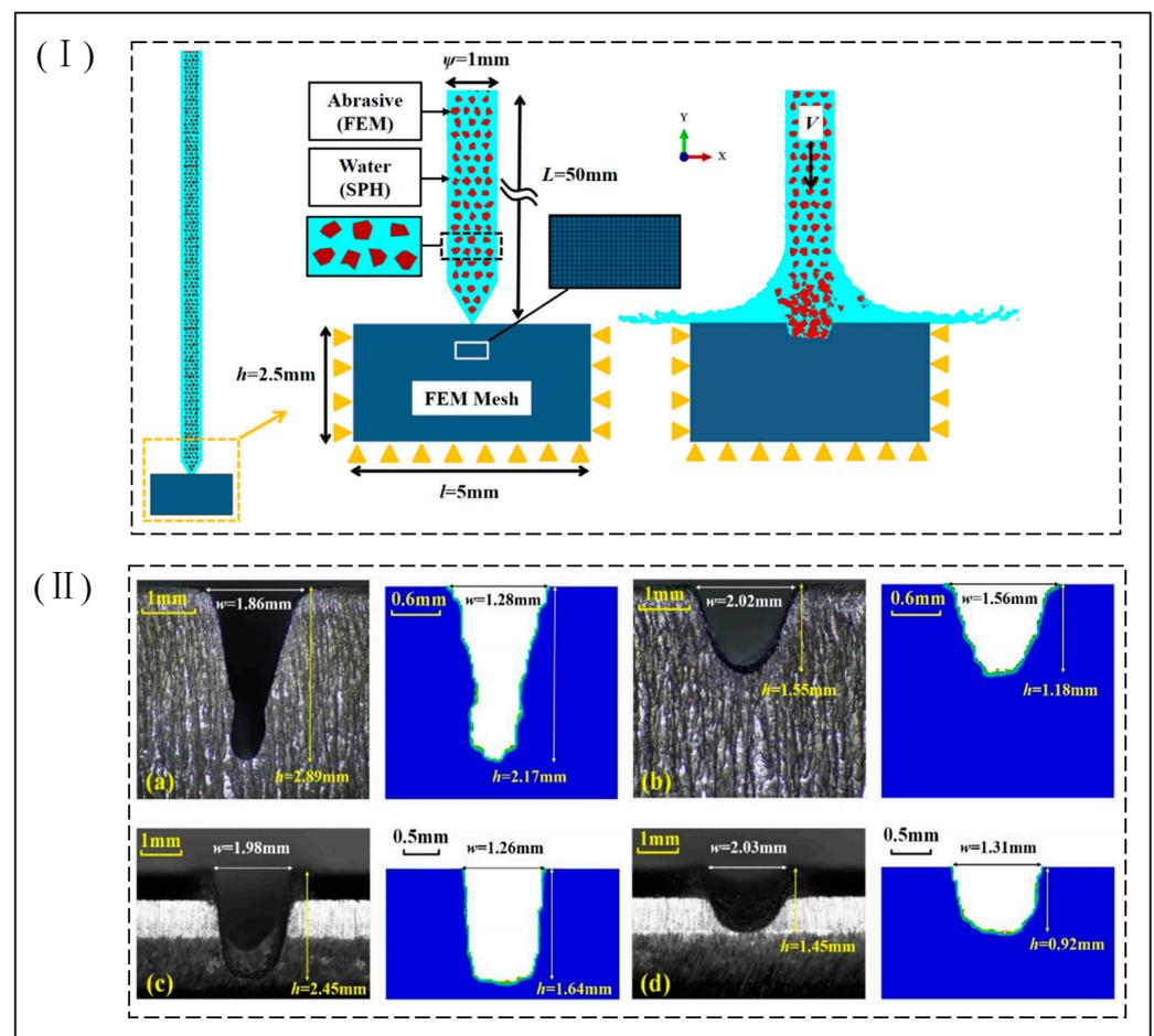
**Figure 8.** Simulation and experiment of abrasive water jet impact on workpieces [58]: (I) FEM-SPH coupled model of abrasive water jet machining material surface; (II) comparison of the experiments and simulations of the kerf profiles under different impact conditions. (a,b) are kerf profiles of Ti6Al4V, and (c,d) are kerf profiles of AISI304.
