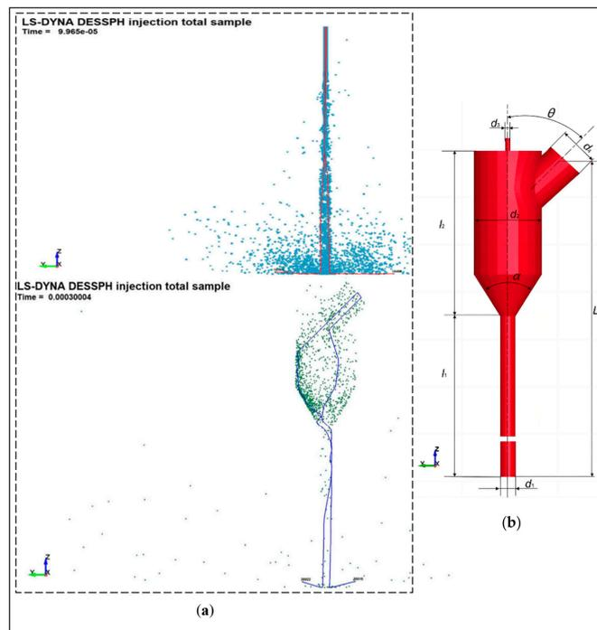
Figure 6. Simulation of abrasive water jet motion processes [47]: (a) the trajectory of the water flow and abrasive particles; (b) geometric modeling of the nozzle.
