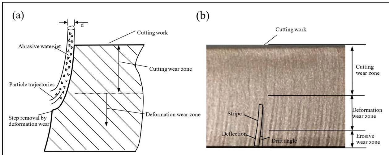
**Figure 3.** (a) formation process of steps in cutting; (b) sectional zoning of cutting actual topography.
