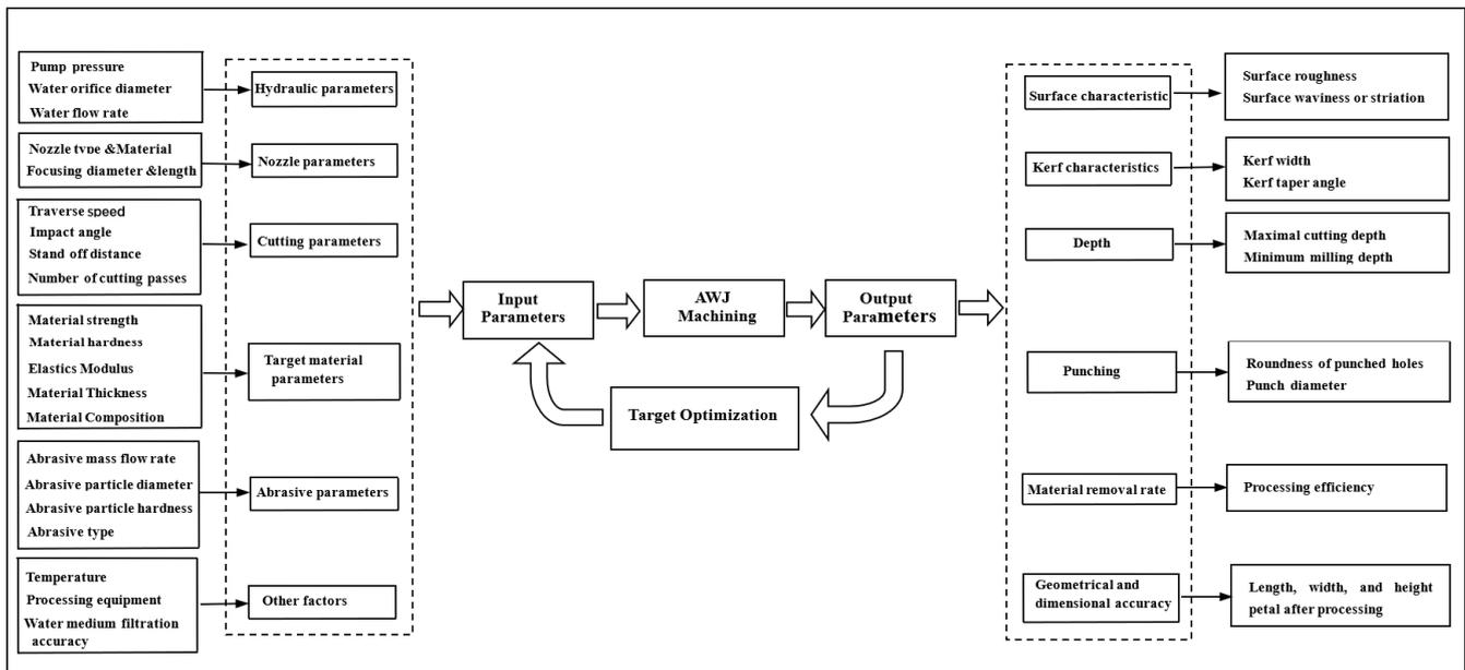
Figure 9. Process parameters influencing abrasive water jet machining.
