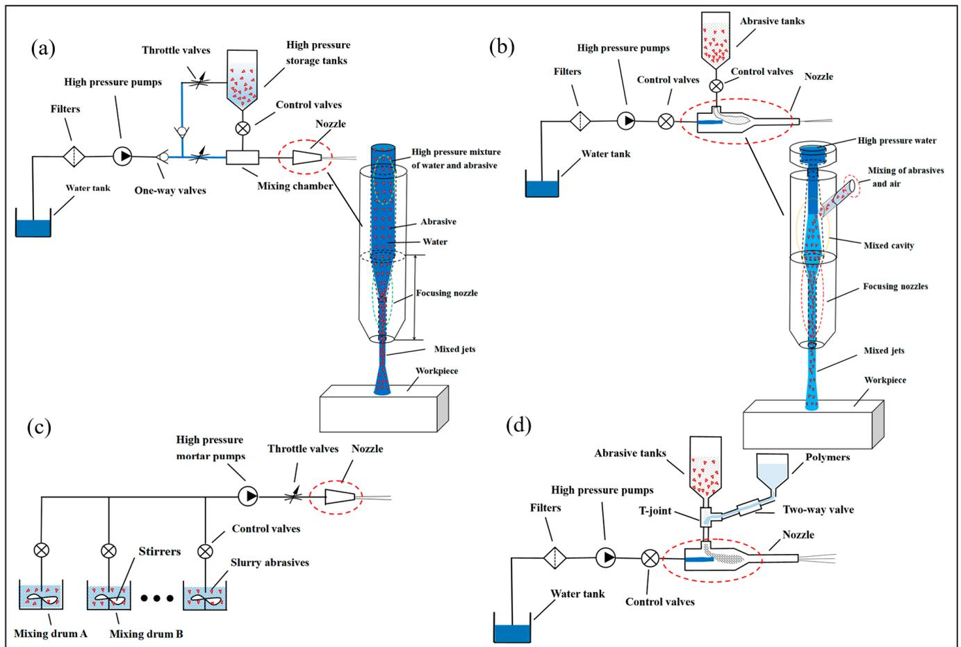
**Figure 1.** Principle diagram of abrasive water jet: (a) Premixed abrasive water jets. (b) Postmixed abrasive water jets. (c) Slurry abrasive water jet. (d) Abrasive water slurry jet.
