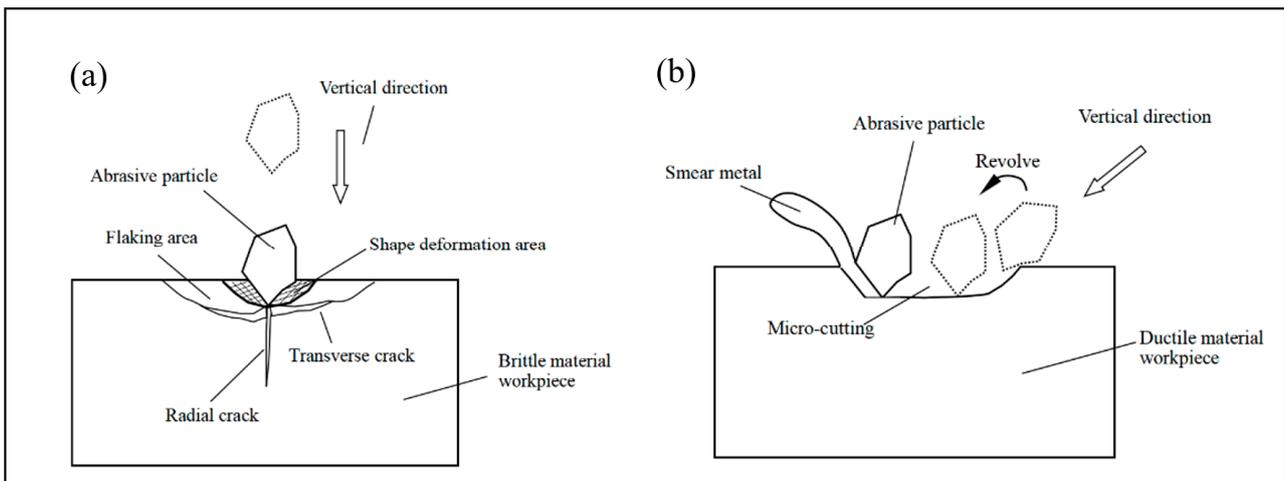
**Figure 2.** (a) damage removal of brittle materials by abrasive particles; (b) damage removal of ductile materials by abrasive particles.
