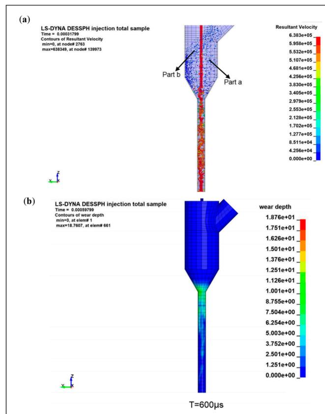
Figure 7. (a) the mixing and accelerating process of abrasive particles in the nozzle; (b) the wear simulation of abrasive waterjet nozzle [47].
