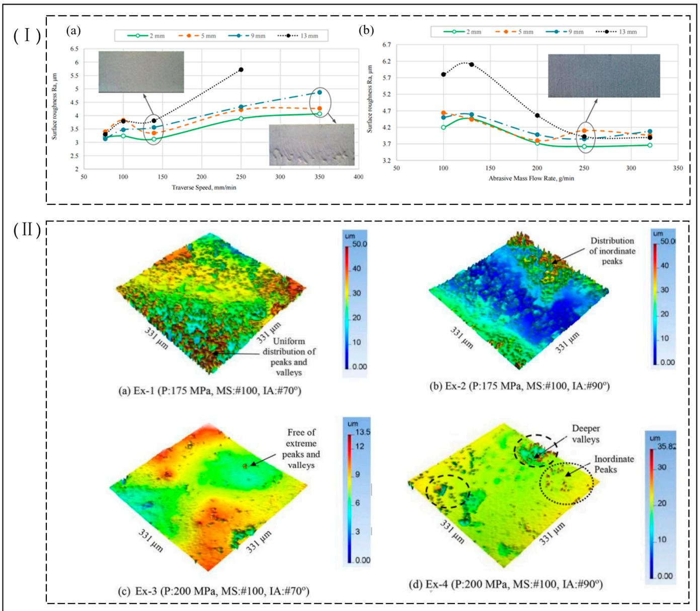
**Figure 11.** (I) effect of process parameters on surface roughness of different cutting areas [69], (a) The effect of traverse speed on the surface roughness on different zones of the cut surface—15 mm thickness; (b) The effect of abrasive mass flow rate on the surface roughness on different zones of the cut surface—15 mm thickness; (II) 3D surface topography at different cutting conditions [80].
