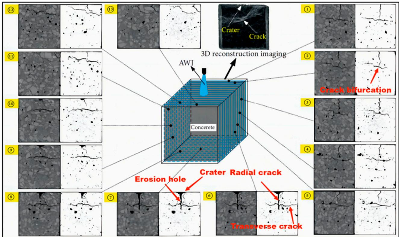
**Figure 4.** The propagation path of cracks in the concrete after abrasive water jet impact in the interior from the distribution and scanning results of CT sections [27]; Serial numbers ①–⑬ represent 13 typical CT slices obtained in the radial direction of the jet.
