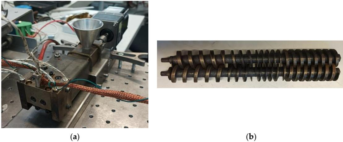
Figure 2. The intermeshing counter-rotating micro-twin-screw extruder: (a) general view of the die, barrel, and drive unit; (b) counter-rotating parallel screws.
