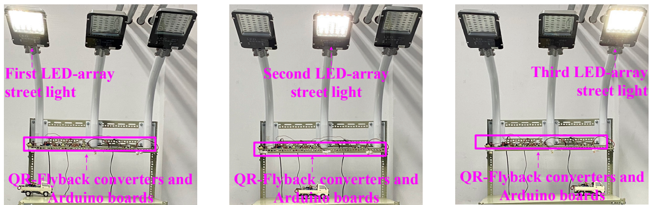
Figure 11. Arduino development board combined with QR-flyback converter to drive LED array streetlamp.
