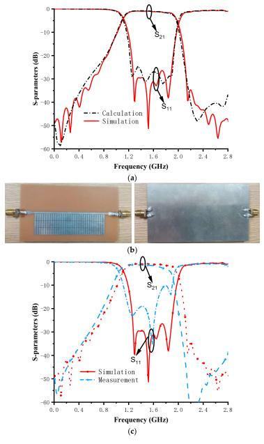
**Figure 5.** (a) Comparison between the calculation and EM simulation results; (b) photographs of the fabricated filter; and (c) comparison between the simulated and measured S-parameters.
