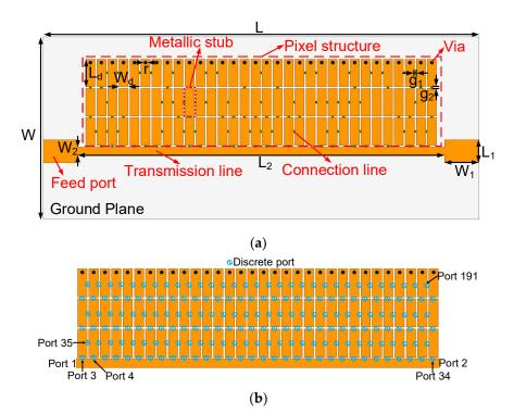
**Figure 1.** Structure of the proposed BPF: (a) layout and (b) definition of port numbers. W = 50, L = 90,  $W_1 = 5$ ,  $L_1 = 3$ ,  $W_2 = 1.5$ ,  $L_2 = 70$ ,  $W_d = 1.8$ ,  $L_d = 6$ ,  $g_1 = 0.2$ ,  $g_2 = 0.2$ , and r = 0.2 (unit: mm).
