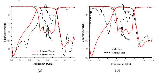
**Figure 2.** Realized S-parameters using different pixel structures. (a) Different sized pixel units and (b) with/without shorting vias.
