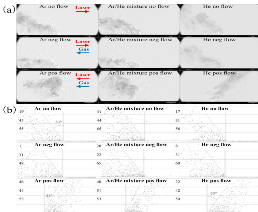
Figure 35. (a) Shadowgraphs extracted at 18,264 ms from the experiments performed under argon, the gas mixture, and helium for the no flow, negative flow, and positive flow configurations; (b) Analysis of the darker (colder) spatters from extracted shadowgraph [167].
