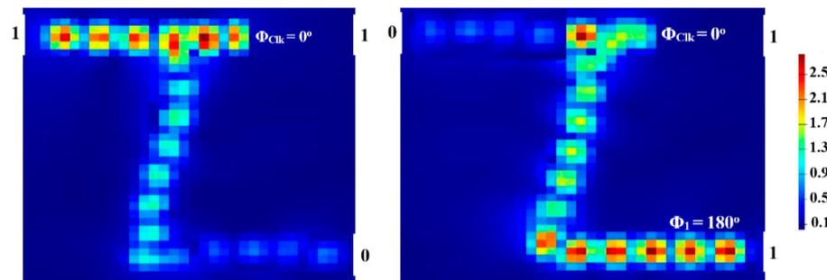
**Figure 9.** NOT field intensity distributions propagating through Z-shaped silicon waveguide at  $1.55 \mu\text{m}$ .
