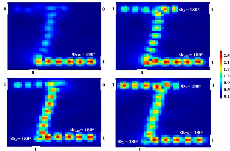
**Figure 8.** OR field intensity distributions propagating through Z-shaped silicon waveguide at  $1.55 \mu\text{m}$ .
