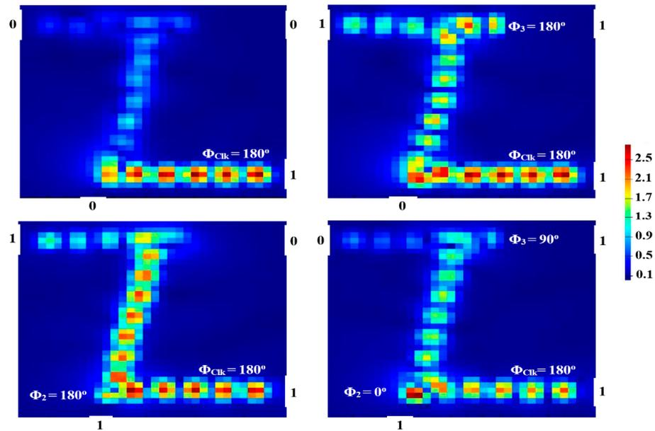
**Figure 6.** XOR field intensity distributions propagating through Z-shaped silicon waveguide at 1.55  $\mu\text{m}$ .
