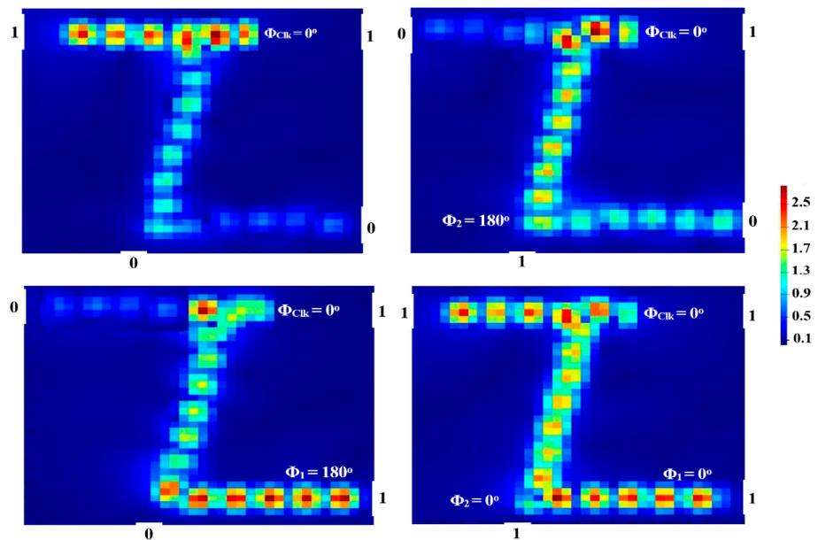
**Figure 12.** XNOR field intensity distributions propagating through Z-shaped silicon waveguide at 1.55  $\mu\text{m}$ .
