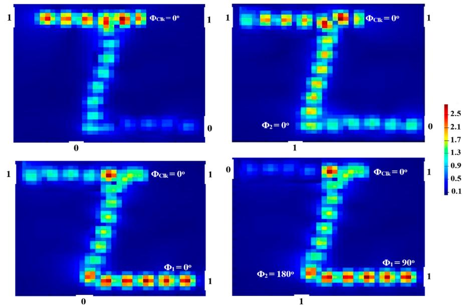
**Figure 11.** NAND field intensity distributions propagating through Z-shaped silicon waveguide at 1.55  $\mu\text{m}$ .
