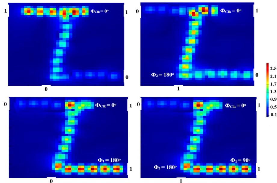
**Figure 10.** NOR field intensity distributions propagating through Z-shaped silicon waveguide at 1.55  $\mu\text{m}$ .
