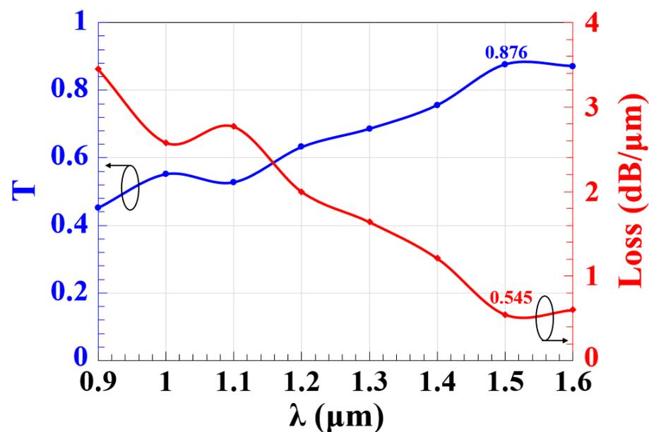
**Figure 2.**  $T$  and loss versus  $\lambda$  employing Z-shaped silicon waveguide.
