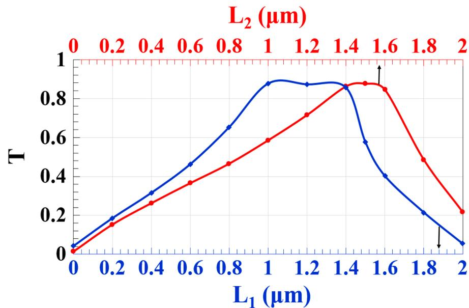
Figure 4. T versus length of the short slot ( $L_1$ ) and length of the long slot ( $L_2$ ) employing Z-shaped silicon waveguide at 1.55  $\mu\text{m}$ .
