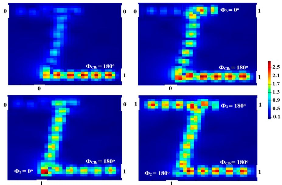
**Figure 7.** AND field intensity distributions propagating through Z-shaped silicon waveguide at 1.55  $\mu\text{m}$ .
