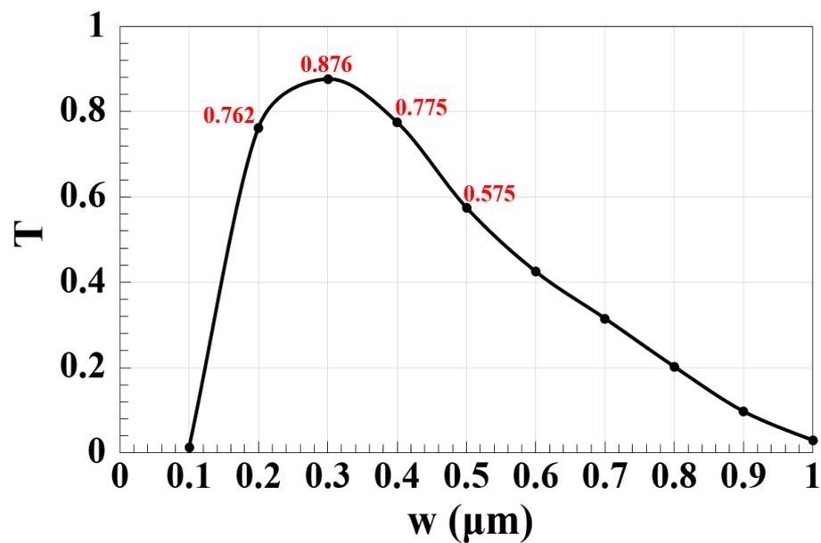
Figure 5. T versus width of the slot (w) employing Z-shaped silicon waveguide at 1.55 μm.
