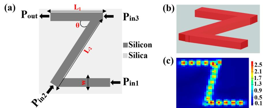
**Figure 1.** (a) Schematic illustration, (b) 3D FDTD view, and (c) field intensity distributions of the Z-shaped silicon waveguide.
