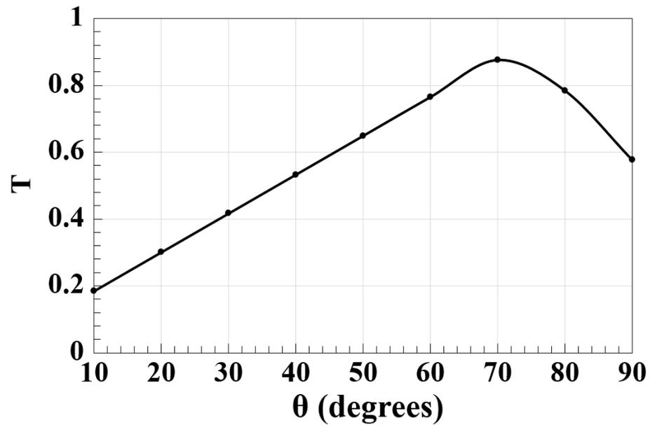
Figure 3. T versus angle between slots ( $\theta$ ) employing Z-shaped silicon waveguide at 1.55  $\mu\text{m}$ .
