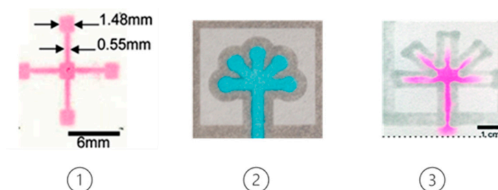
Figure 8. ① Using inkjet printing of poly(styrene) with toluene and colored ink, to visualize the paper's structure. Reproduced with permission from Ref. [85] 2008 American Chemical Society. ② Micro-PADs fabricated via printing a pattern on chromatography paper with an ink-jet printer. Reproduced with permission from Ref. [82] PMC Open Access Subset. ③ Hydrophilic channels can be created on paper by printing hydrophobic PDMS, followed by introducing a 10- \mu L sample into the channels. Reproduced with permission from Ref. [103] © 2023 Copyright American Chemical Society.
