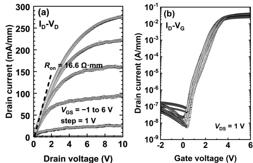
Figure 3. (a) Output and (b) transfer characteristics of the ITO-gated p-GaN gate HEMTs at room temperature.
