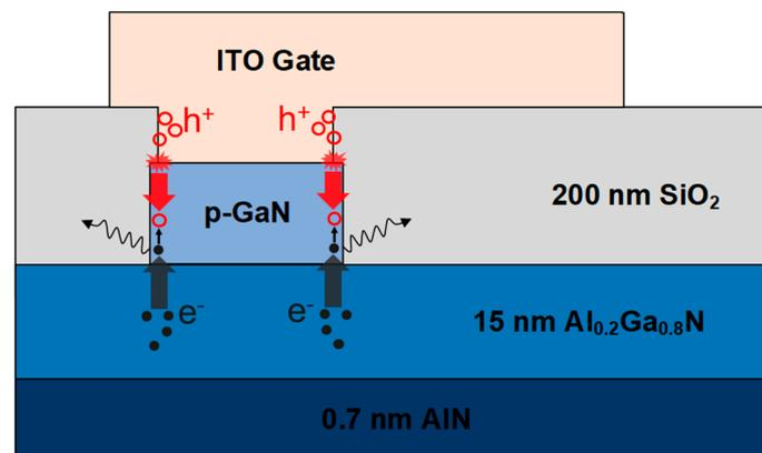
**Figure 7.** Gate failure and luminescence mechanism of the p-GaN gate HEMTs.
