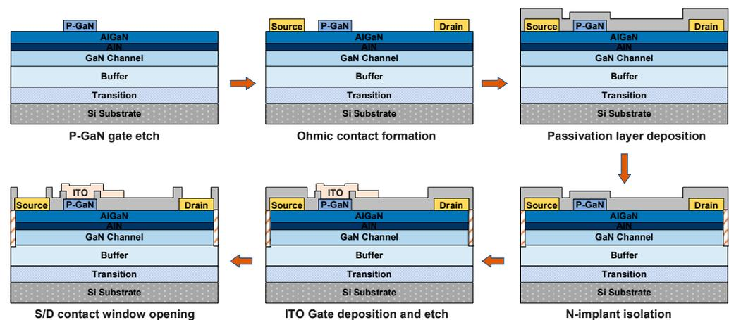
Figure 2. Simplified fabrication process of the ITO-gated p-GaN gate HEMTs.
