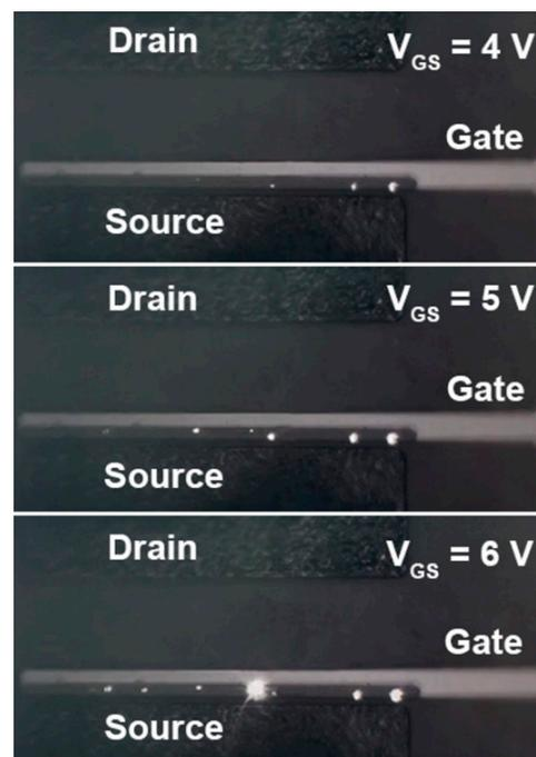
**Figure 6.** Photos of ITO-gated p-GaN gate HEMTs luminescence under  $V_{DS} = 0$  V and various  $V_{GS}$  after gate failure.
