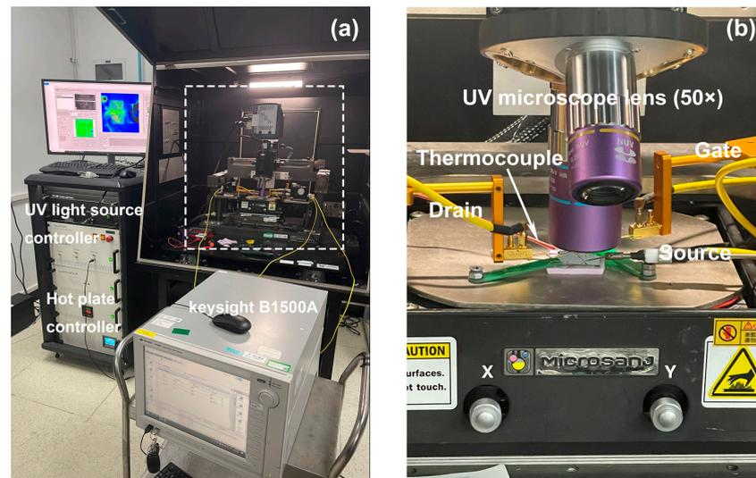
**Figure 4.** (a) The thermal reflectivity imaging system, including electrical measurement, heat measurement, and reflectance calibration section. (b) The details of the system dotted box in (a).
