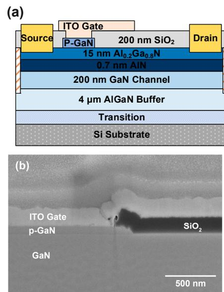
**Figure 1.** (a) Cross-sectional diagram of a p-GaN gate HEMTs with an ITO gate. (b) FIB-SEM photograph of the device's gate stack as well as the gate field plate above the  $\text{SiO}_2$  passivation layer.
