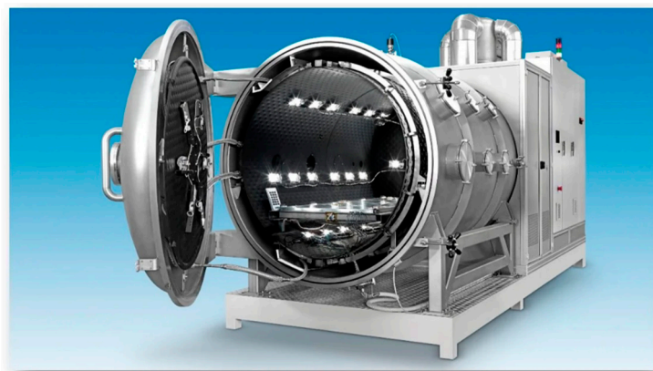
Figure 6. The thermo-vacuum chamber employed in the tests.
