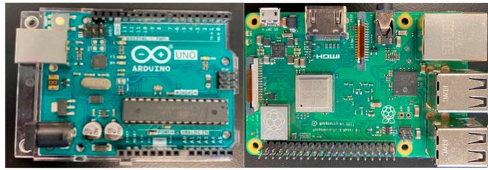
**Figure 3.** Commercial data processors Arduino UNO (**left**) and Raspberry Pi (**right**).
