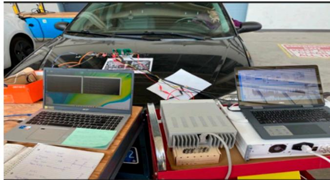
**Figure 4.** The experimental test setup to measure the dynamic data of the sedan vehicle.
