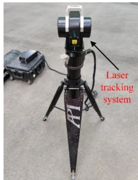
Figure 8. Deformation measurement system.
