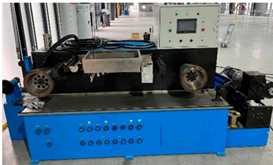
**Figure 19.** Tungsten wire drawing equipment.
