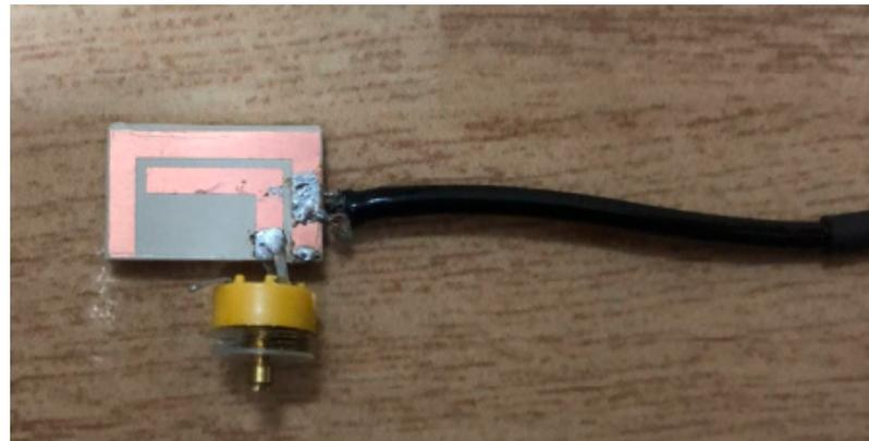
**Figure 7.** The fabricated prototype of the planar inverted L-C antenna.
