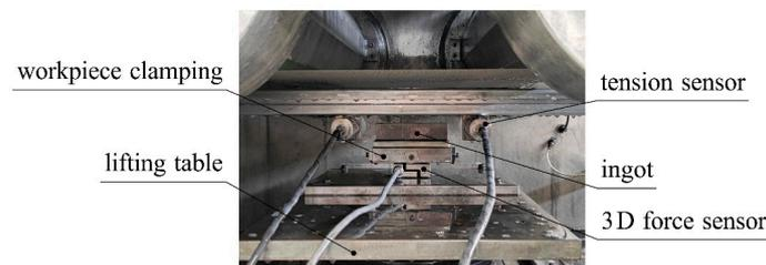
Figure 20. Physical diagram of the experimental platform.
