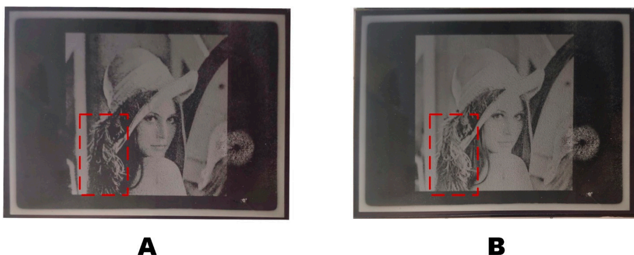
Figure 17. The picture of “Lena” displayed on the EWD, the red rectangles show the difference between the two different waveforms. (A) Display with the +15 V DC waveform. (B) Display with the proposed multi-DC waveform.
