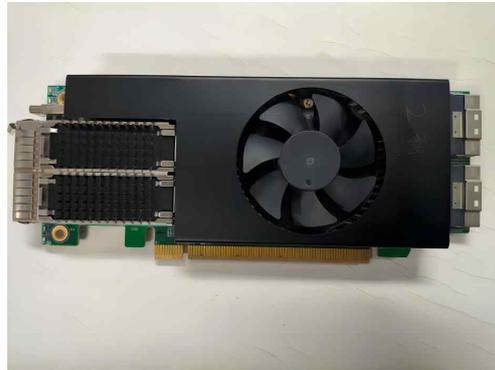
**Figure 5.** TCP Offload Engine (TOE) on FPGA chip.
