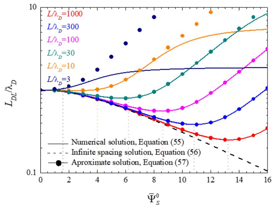
**Figure 3.** Dependence of the electric double layer thickness values on the surface potential, calculated for the indicated  $L/\lambda_D$  values. Vertical dot lines show surface potential values corresponding to the double layer thickness minima, Equation (58).
