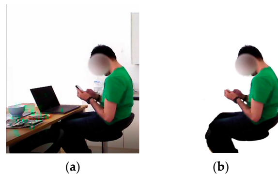
Figure 3. (a) Before background deduction and (b) after background deduction of a frame sequence from HWU-USP dataset.
