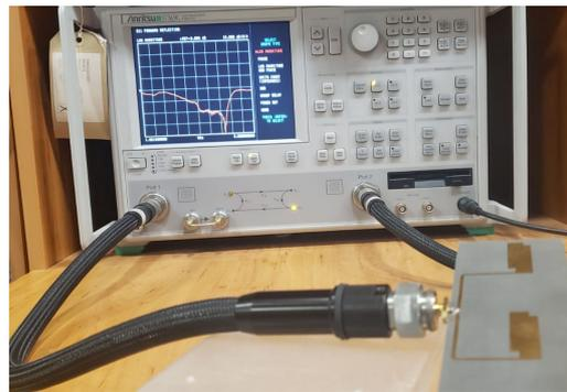
**Figure 4.** The reflection coefficient and input impedance measurement setup.
