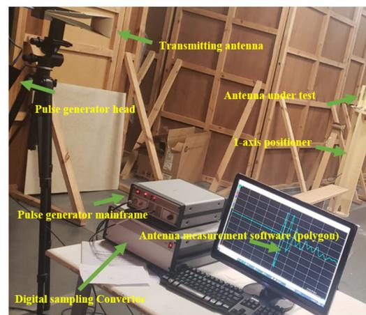
**Figure 5.** Geozondas time-domain antenna measurement setup.
