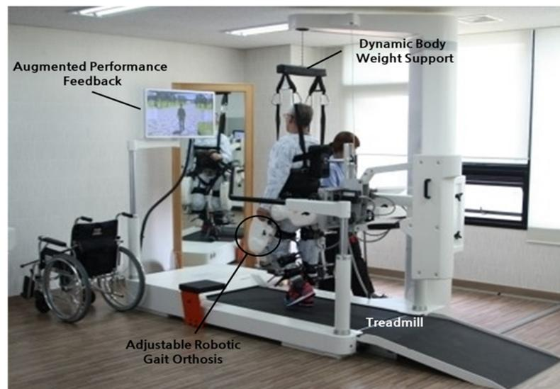
**Figure 14.** Lokomat device used for gait rehabilitation following lower-limb disability, brain injury, or spinal cord injury. The device consists of a treadmill, body weight support, and powered leg orthosis [70].
